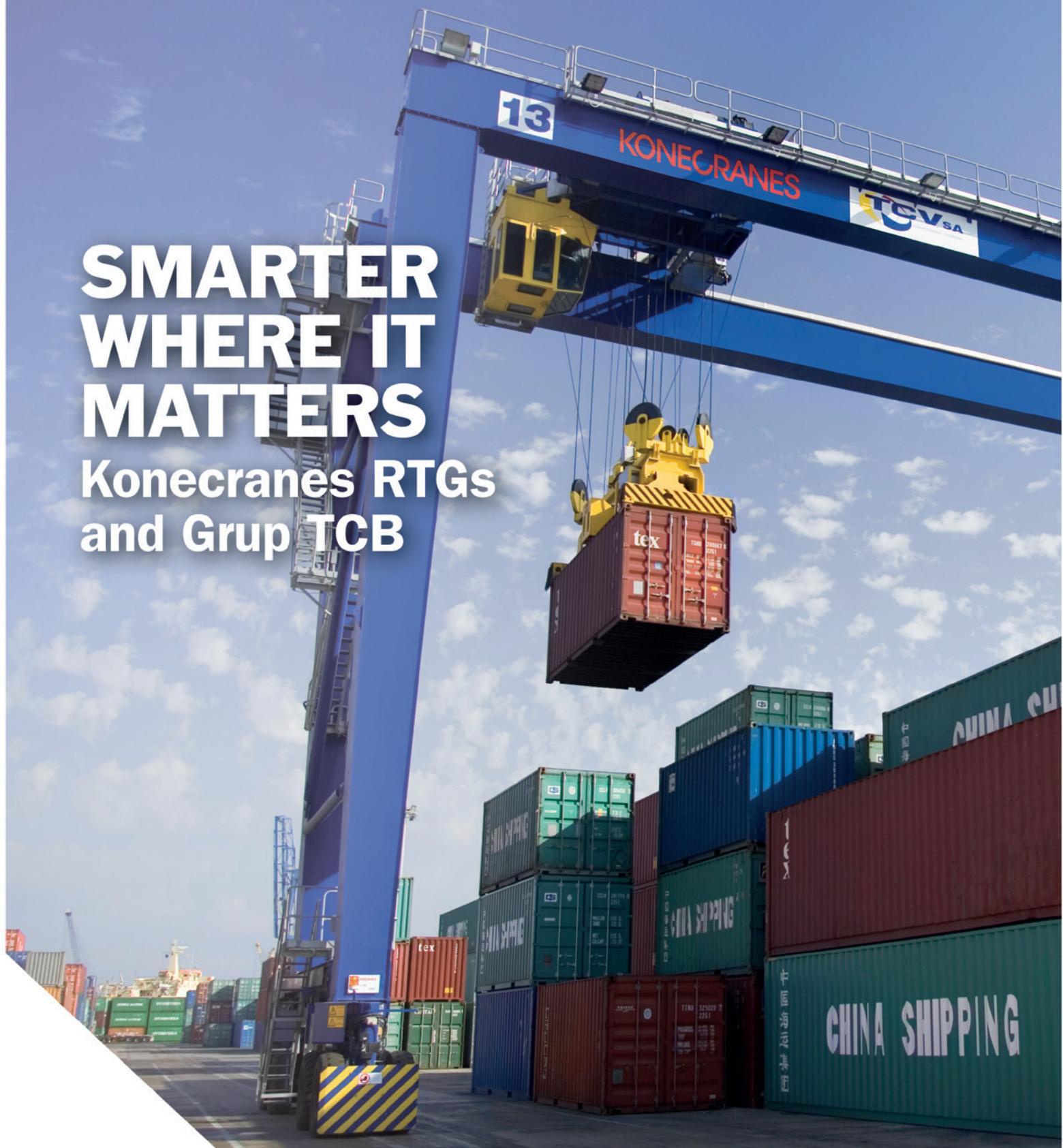
Grup TCB operates 35 Konecranes RTGs at four container terminals around the world. Here you see a Konecranes 16-wheel RTG at work in Grup TCB's container terminal in Valencia, Spain. Thanks to its Active Load Control system and the smart design of its steel structure, this is a very productive crane.
